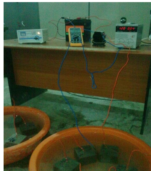
Figure 2: Electrical connection for applying a +12 V fixed anodic potential to accelerate the corrosion
