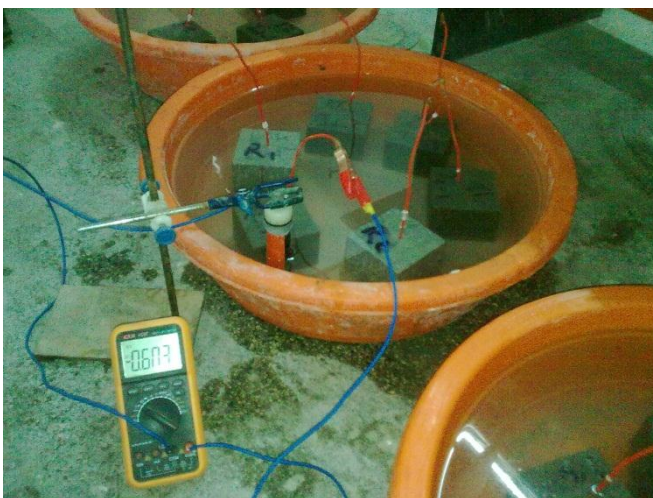
Figure1: corrosion potential measurement
