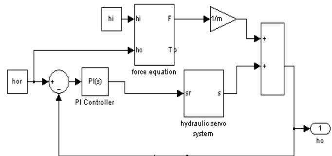
Fig.9: Simulink model of the strip thickness control.
