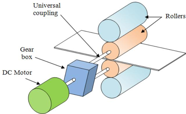
Fig.6: The main drive system of rolling mill.
