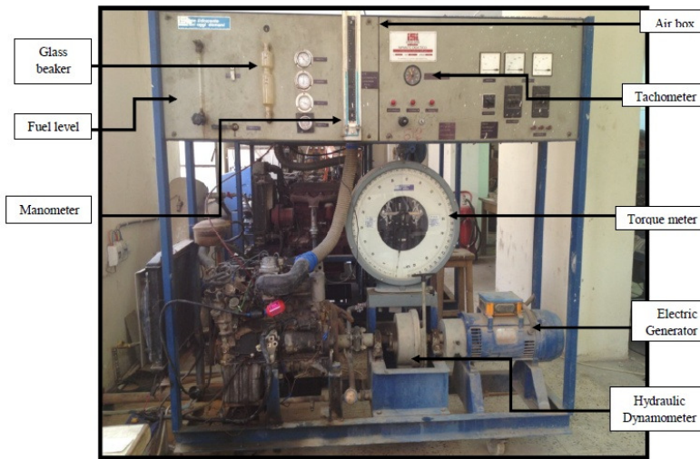
Fig. 1. The experimental rig of SI engine.
