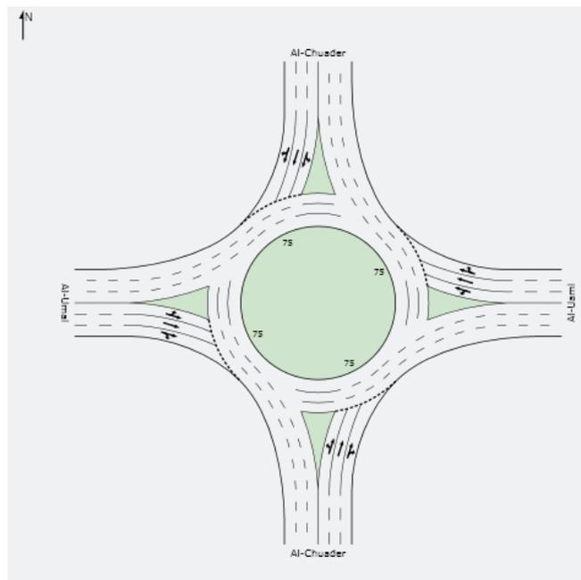
**Fig. 2. Sidra layout image for Mudaffar roundabout.**
