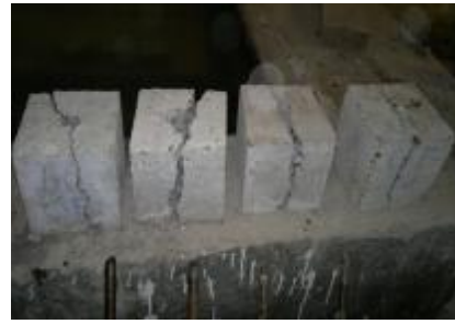
Figure (10) Splitting Failure.
