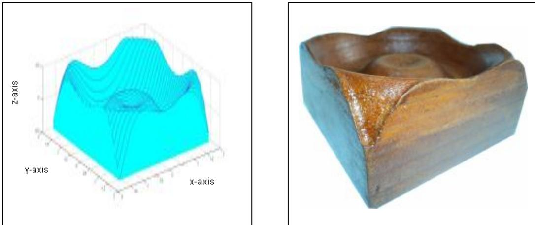
Figure (15) a- Tool path of the 3<sup>rd</sup> Sculptured Surface. b- Machined Surface
