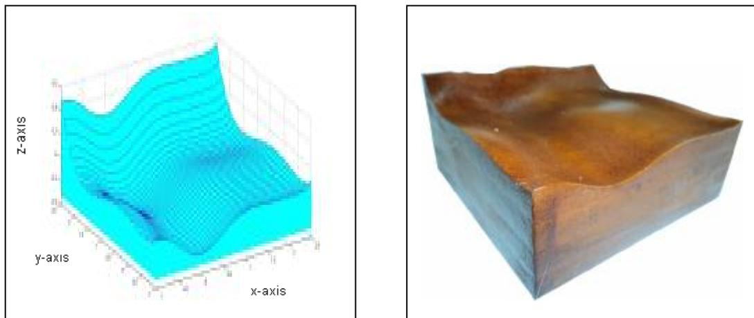
Figure (14) a- Tool path of the 2<sup>nd</sup> Sculptured Surface. b- Machined Surface
