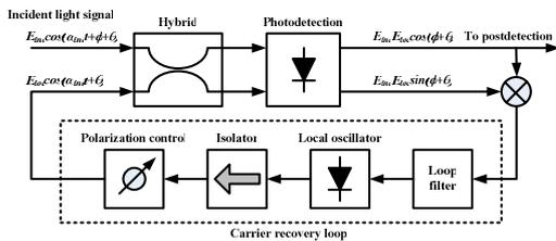
Fig. (2) Block diagram of homodyne coherent detection
