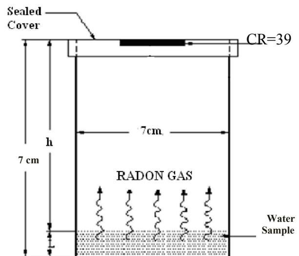
Fig.2 Experimental setup for measurements of radium and radon concentrations in water samples.
