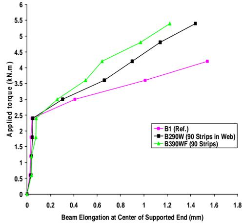
Figure (12) Beam Longitudinal Elongation Behavior: Effect of Flange Strengthening
