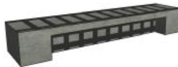
Fig (5) Strengthened Beam with 90° CFRP Strips in the Web and Flange and Longitudinal CFRP in the Web and Flange (B690WFL)
