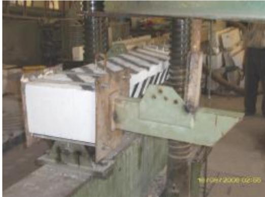
Figure (8) Clamping Torsional Arm
