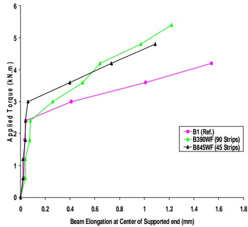
Figure (16) Beam Longitudinal Elongation Behavior: Effect of Fiber
