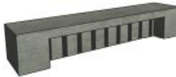
Fig (3) Strengthened Beam with 90° CFRP Strips in the Web Only (B290W)
