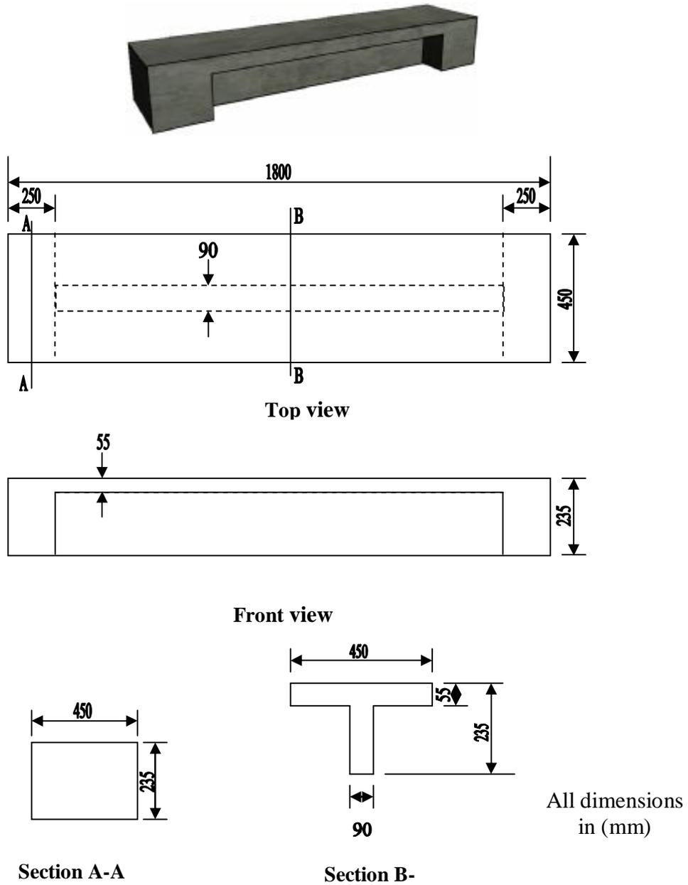
Figure (1) Beam Specimen with Dimensions
