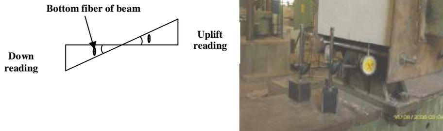
Figure (10) Angle of Twist Measurement
