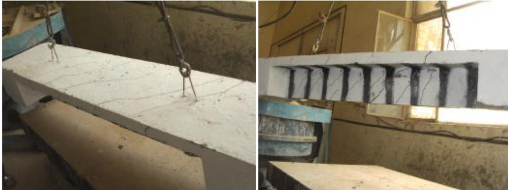
Figure (13) Mode of Failure of Strengthened Beam B290W (90° Strips in the Web Only)
