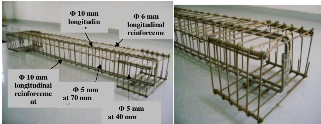
Figure (7) Details of Beam Reinforcement
