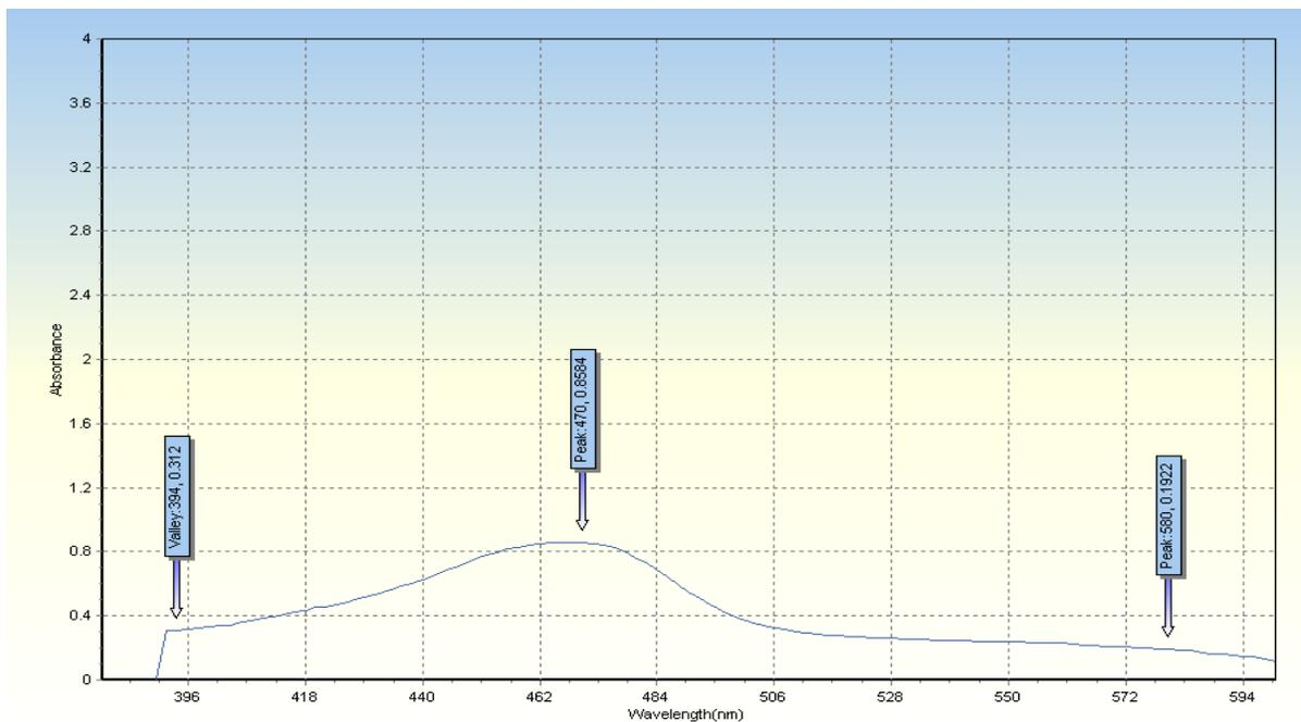
**Fig. (3):- Absorption spectrum of MD-NBD-Cl system against reagent**
