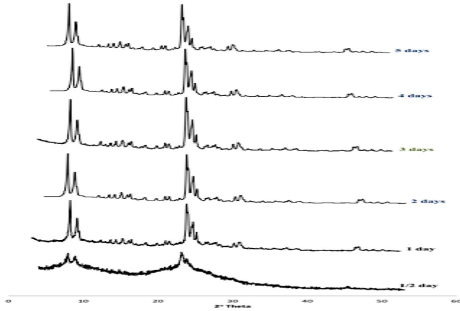
Figure 1. XRD patterns for the ZSM-5 zeolites at different crystallization times.
