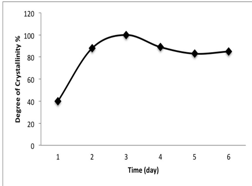
Figure 2. Crystallization times effect on the degree of the crystallinity for the ZSM-5.
