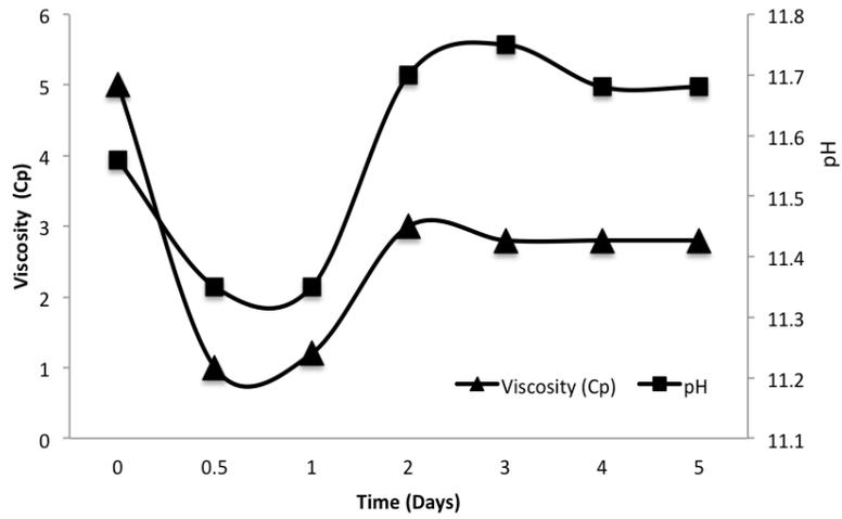
Figure 3. pH and viscosity variation of the reaction gel with the crystallisation time.
