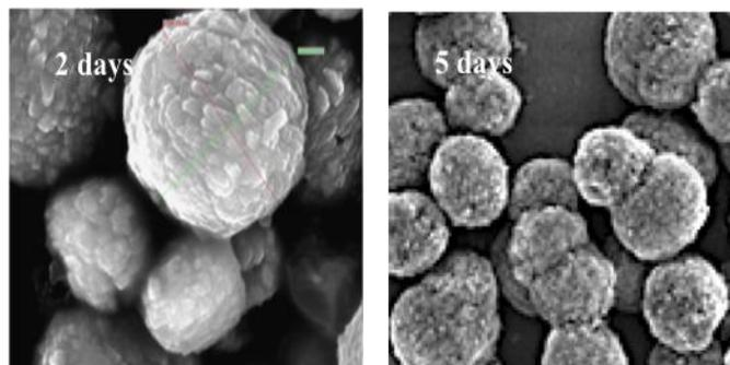
Figure 5. ZSM-5 crystal size at different crystallization times.
