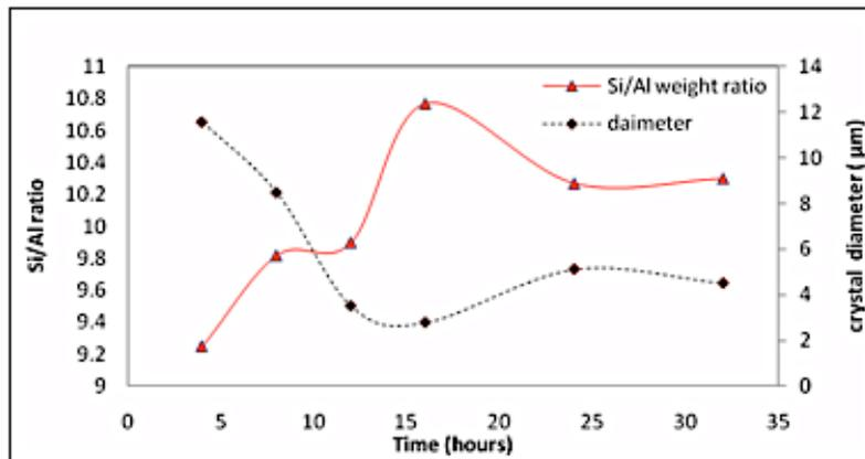
Figure 8. Effect of ageing time on the crystal size, Si/Al bulk ratio.
