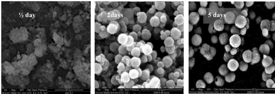
Figure 4. ZSM-5 morphology at different crystallization times.
