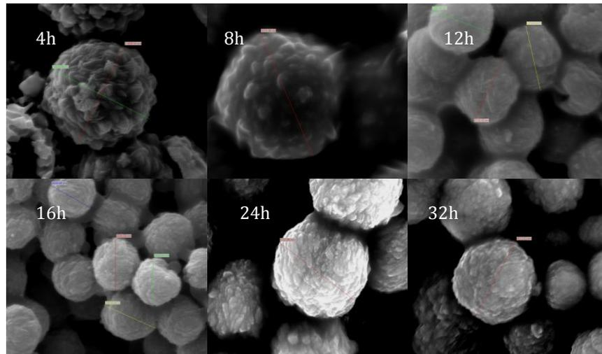
Figure 7. ZSM-5 crystal size at different ageing times.
