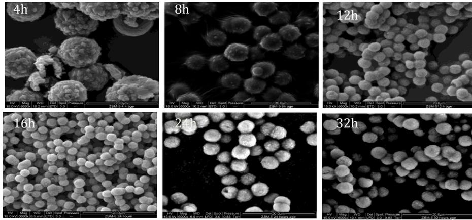
Figure 6. SEM images of ZSM-5 for different ageing times.
