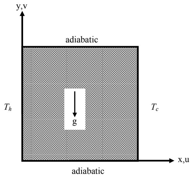
**Fig. 1 Schematic diagram of the physical model and coordinates system**
