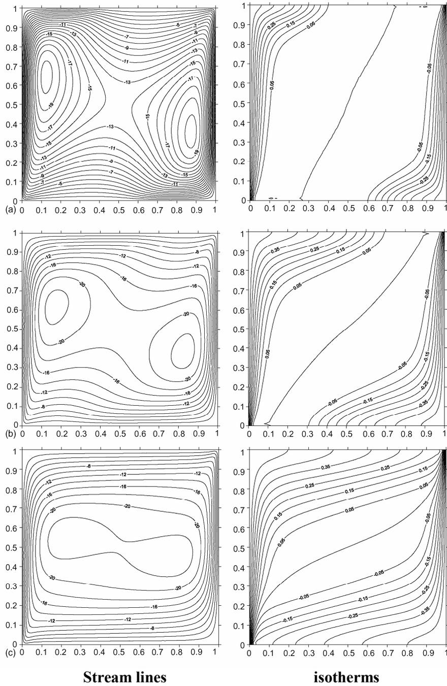
Fig. 2. Stream lines and isotherms for  $Ra = 1000$ ; (a) and  $\tau = 0.0025$ , (b) and  $\tau = 0.005$ , (c)  $\tau = 0.01$ ,
