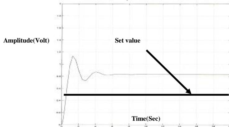
Figure (12) Step response when gain=5 and set value=0.5 with velocity feedback
