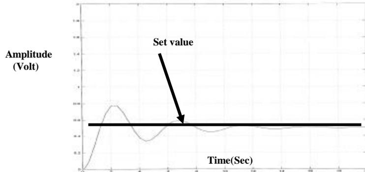
Figure (8) Step response when gain=1 and set value=0.5 without velocity feedback
