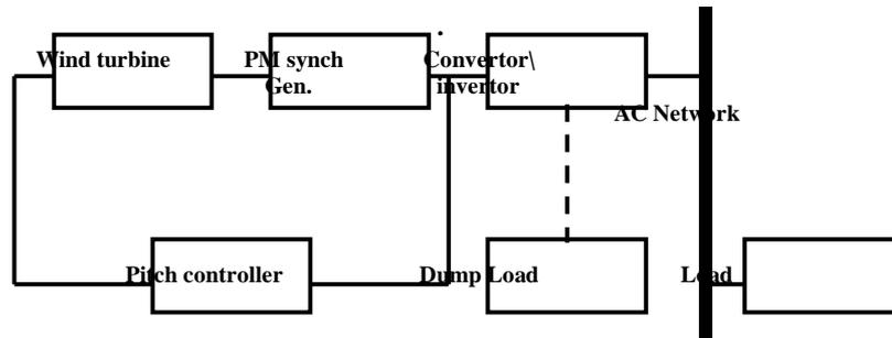
Figure (2) Block diagram of standard variable speed wind generator based system
