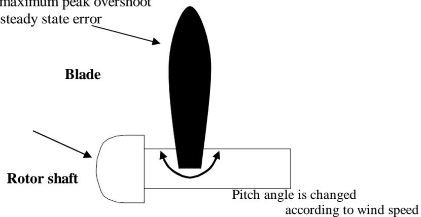
Figure (1) Side view of turbine blade
