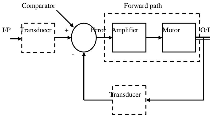
Figure (15) Elements of a closed-loop system
