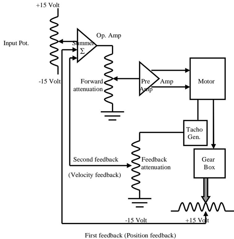
Figure (4) Circuit diagram for position control system
