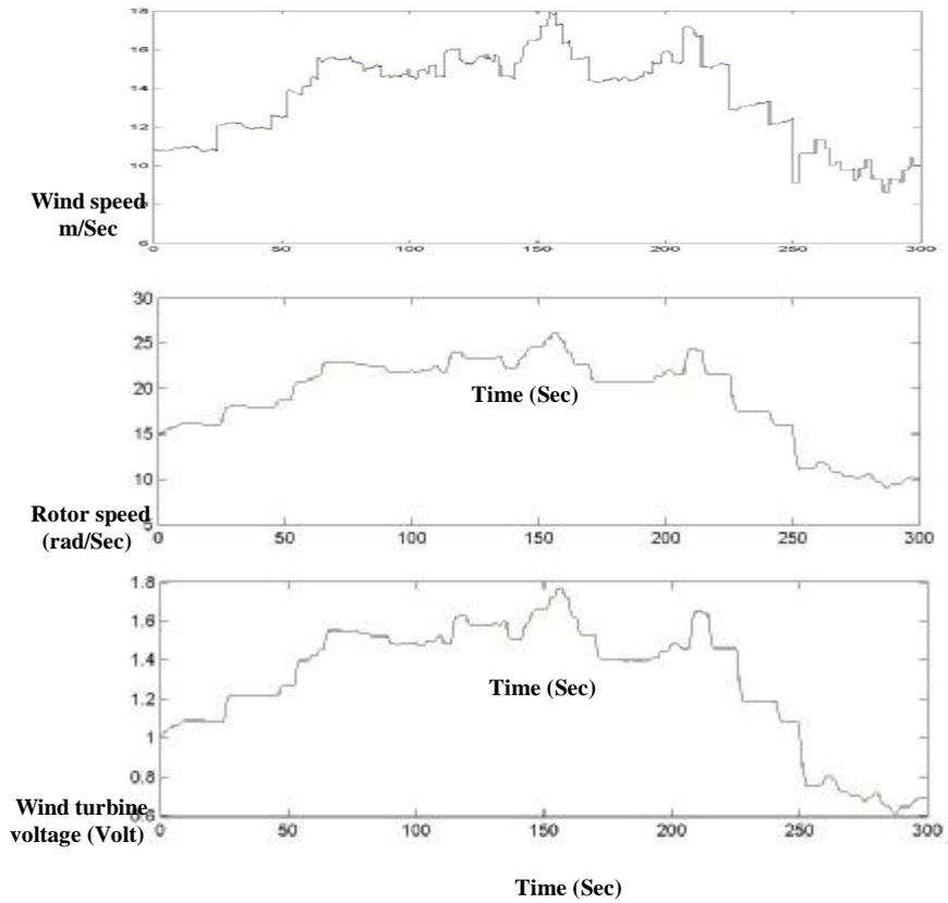
Figure (6) Wind speed, rotor speed and output voltage (uncontrolled)
