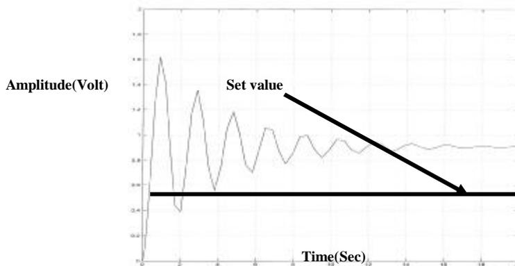
Figure (10) Step response when gain=10 and set value=0.5 without velocity feedback
