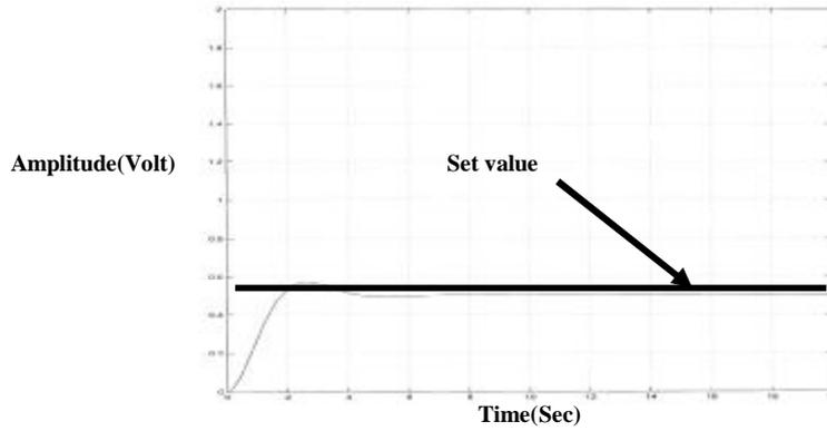
Figure (11) Step response when gain=1 and set value=0.5 with velocity feedback
