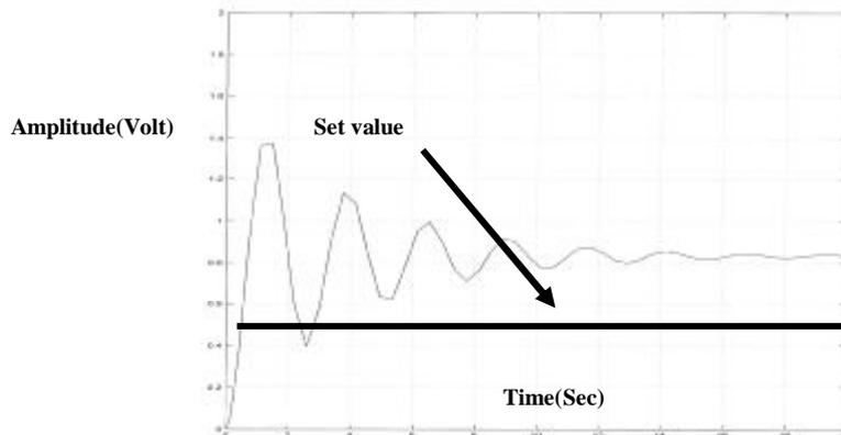
Figure (9) Step response when gain=5 and set value=0.5 without velocity feedback
