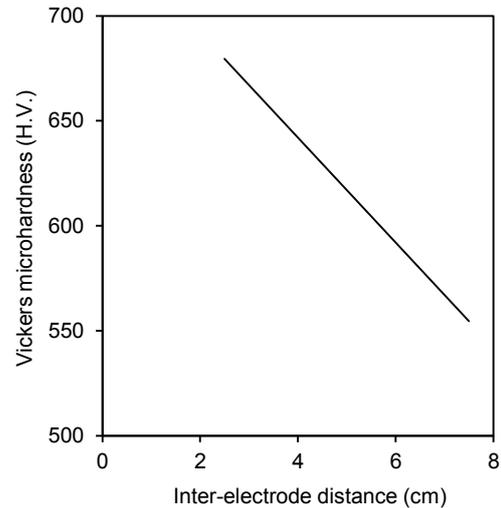
**Fig. (4) Vickers microhardness of the prepared silicon nitride thin films as a function of inert-electrode distance**
