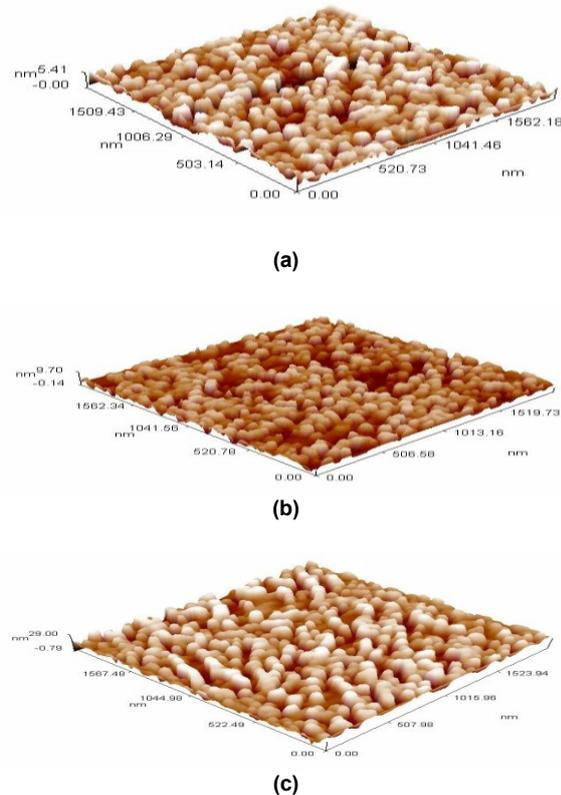
**Fig. (4) 3D AFM of the silicon nitride nanostructures prepared at 1:1 mixing ratio of Ar:N<sub>2</sub> and inter-electrode distance of (a) 2.5, (b) 4.5 and (c) 7.5 cm**
