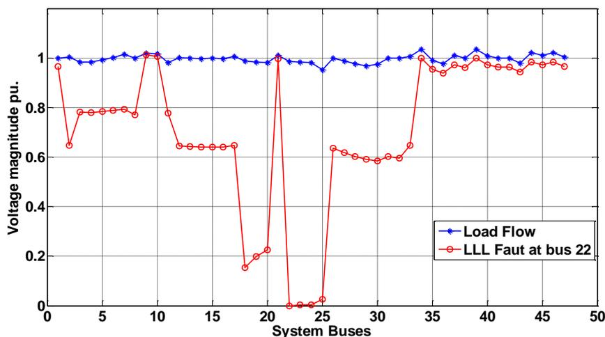
Fig.4 Bus voltage magnitudes before and after LLL fault in Bus 22
