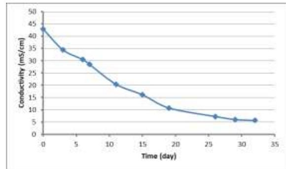
Figure 3: Variation of water conductivity in the desalination chamber with time
