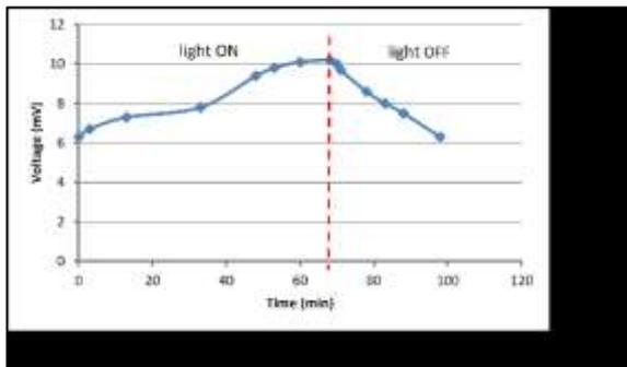
Figure 7: Performance of microalgae biocathode MDC, R=230 Ω.
