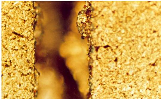
**Fig. (18) The crack propagation through the composite itself (X 10).**
