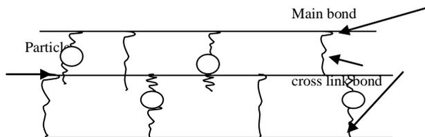
**Fig. (8) The model for particles location inside intermolecular spaces.**
