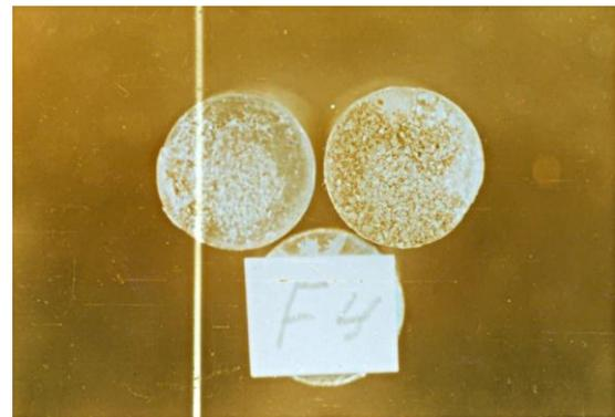
**Fig. (15) The composite adhesive specimen for 60%EP/40%Fe the fracture growth from the interface through the adhesive (X 10).**
