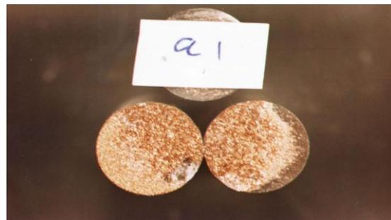
**Fig. (10) The composite adhesive 90%EP/10%Cu (X 10).**
