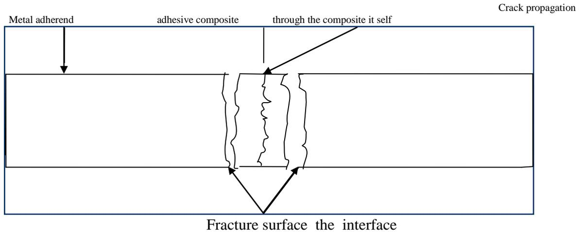
**Fig. (16) The expected mechanism for the crack propagation in adhesive tensile specimen tests.**
