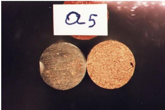
**Fig. (12) The composite adhesive 90%EP /10%Cu ( X 10).**
