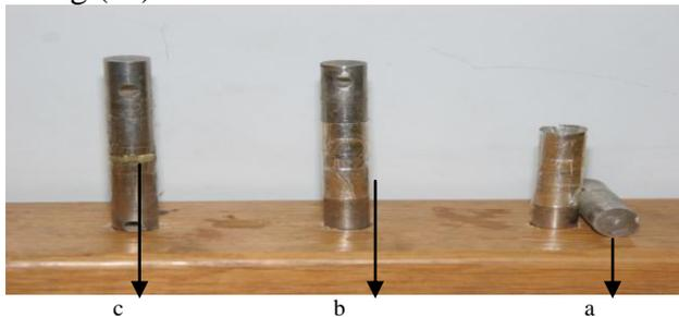
**Fig. (1) Steps of preparation of adhesion sample**
