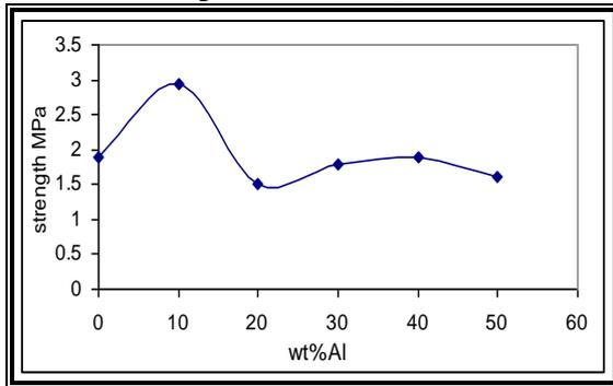
Fig. (4) The strength v.s wt% for EP /Al composites adhesive.
