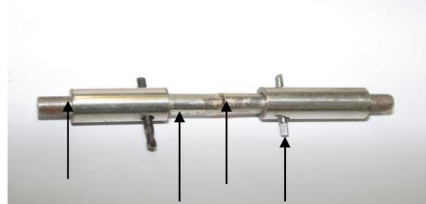
**Fig. (2) Adhesion test sample with holders**
