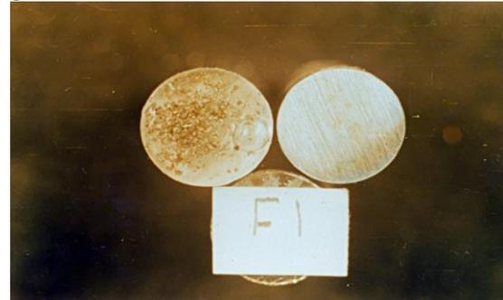
**Fig (14) composite adhesive specimen for 90%EP /10%Fe (X10)**
