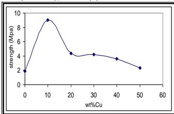
Fig. (5) The strength v.s wt% for the EP /Cu composite adhesive.
