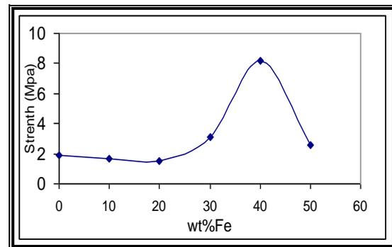
Fig. (6) The strength v.s wt% for the EP /Fe composite adhesive
