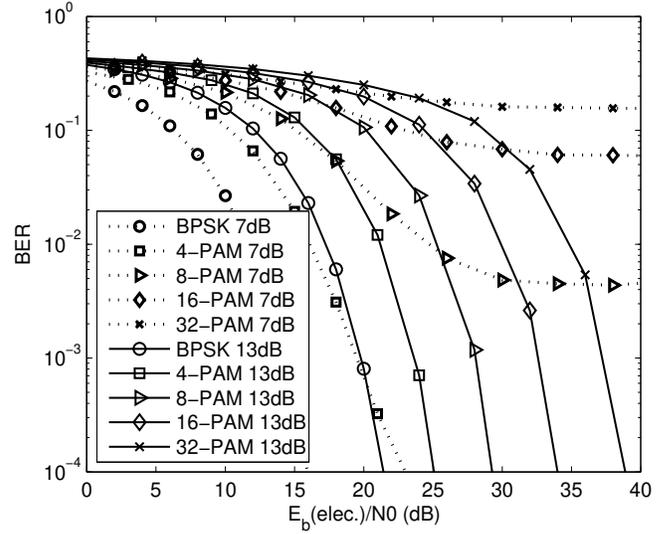
Fig. 2. BER performance of DC-biased IM/DD optical DHT-OFDM system over AWGN channel.
