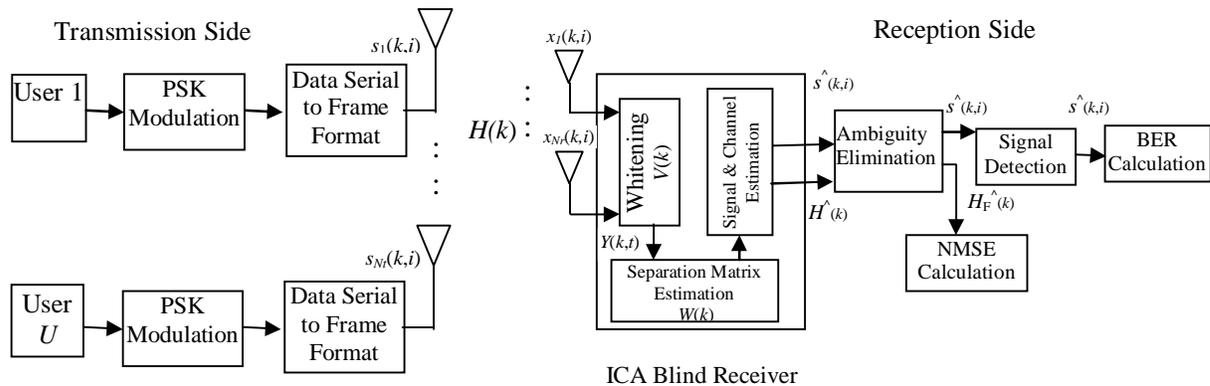
Fig. 1. The Proposed Multiuser CDMA System with Blind Receiving System based on ICA
