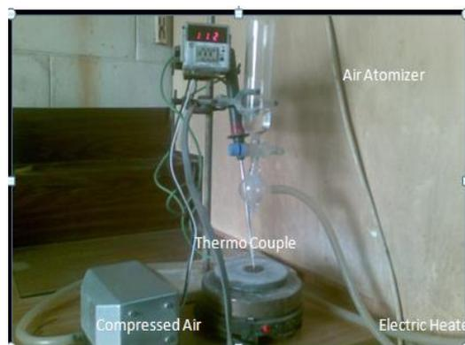
Fig. (4) The air atomizer set up system.
