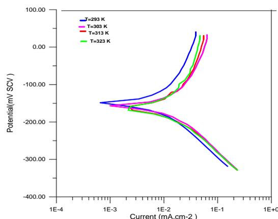
**Fig. (11) shows the polarization curves of stainless steel coated with ZnO at different temperatures.**
