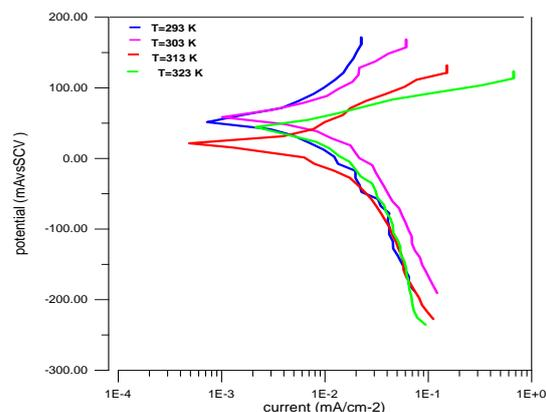
**Fig. (10) shows the polarization curves of stainless steel coated with Al<sub>2</sub>O<sub>3</sub> at different temperatures.**
