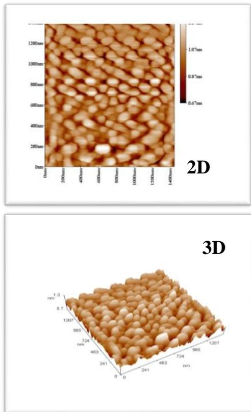
Fig.(6) 2D and 3D views of AFM image of Al<sub>2</sub>O<sub>3</sub>-NaSiO<sub>2</sub> nanoparticles applied on stainless steel.
