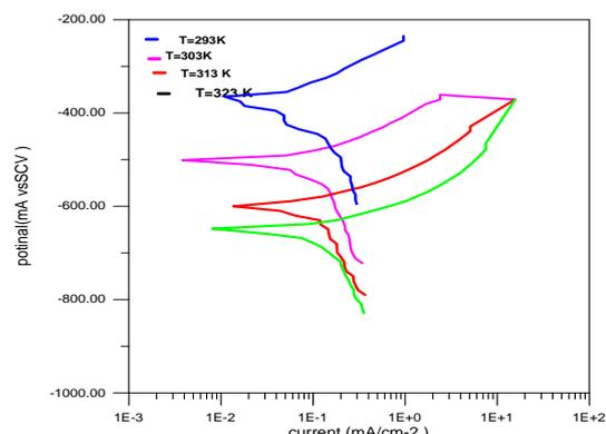
Fig.(8) shows the polarization curves of uncoated carbon steel at different temperatures.
