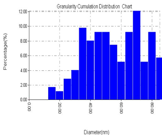
Fig.(7) view of granularity normal distribution chart of Al<sub>2</sub>O<sub>3</sub>-NaSiO<sub>2</sub> nanoparticles.
