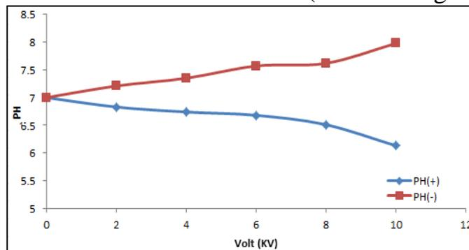
**Figure 3** - Variation of the PH value for distilled water with the applied voltage of both positive (blue line) and negative (red line) corona discharges.
