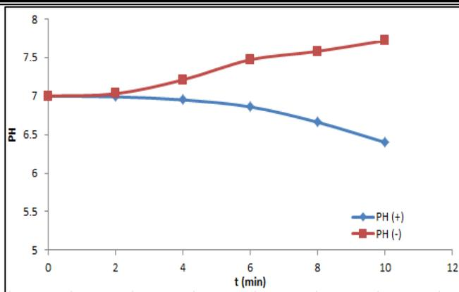
**Figure 6** - The effect of corona discharge on the PH - time relationship of the distilled water in positive corona (blue line) and negative corona (red line).
