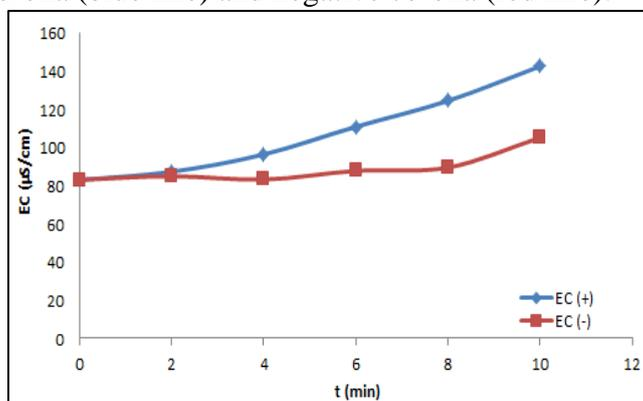
**Figure 8** - The effect of corona discharge on EC - time relationship of the distilled water in positive corona (blue line) and negative corona (red line).
