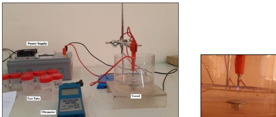
**Figure 2** - The photograph of the electrical discharge system.
