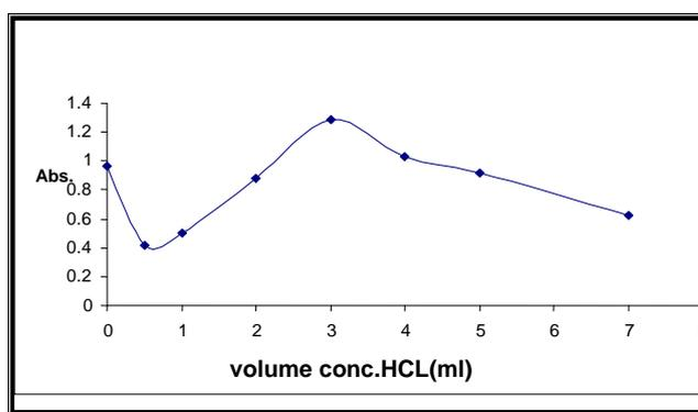
**Fig.(3):** best volume of concentrated hydrochloric acid for determination of paracetamol.
