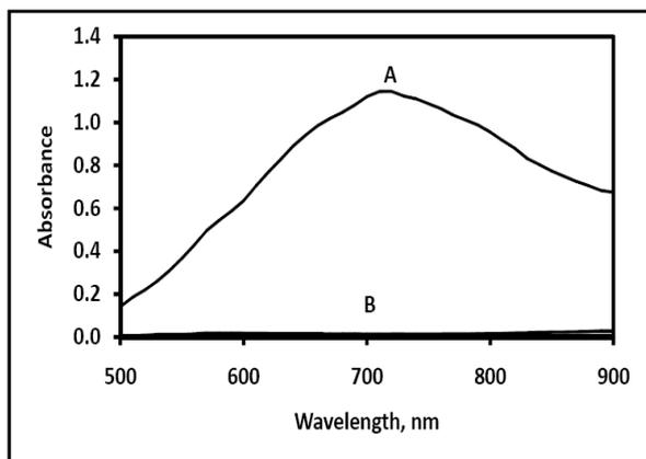
**Fig. (1):** Absorption spectra of A ( $5 \mu\text{g mL}^{-1}$ ) of paracetamol treated as described under procedure and measured against a reagent blank and B the reagent blank measured against distilled water.
