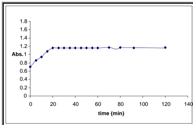
Fig.(4): effect of time (min) on absorbance for determination of paracetamol.
