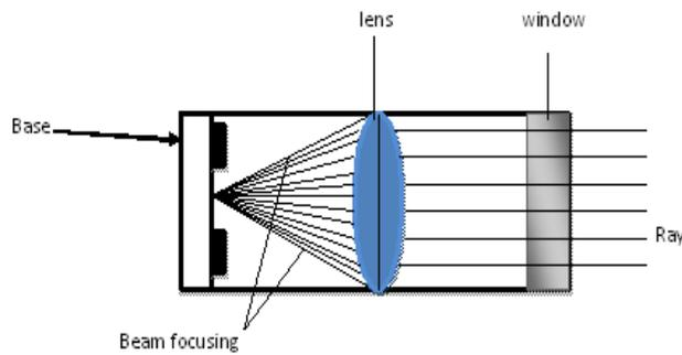
Figure (5) The component of head detector .
