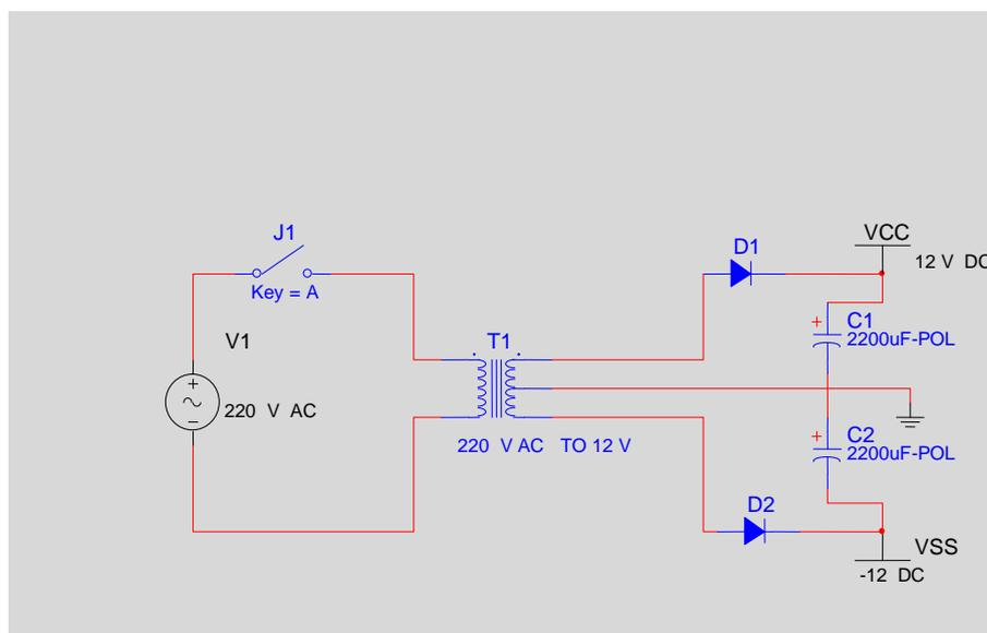
Figure (7) show power supply for tracking circuit.
