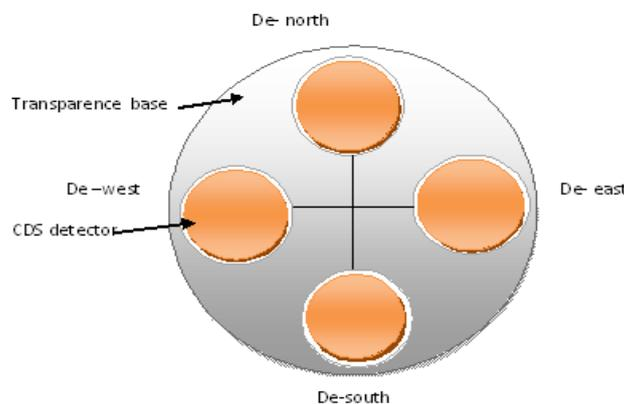
**Figure (4) Distribution of CdS detector on a sensor head**
