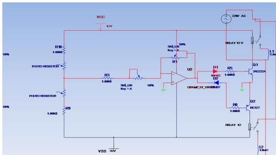
Figure (6) show circuit diagram for tracking system.
