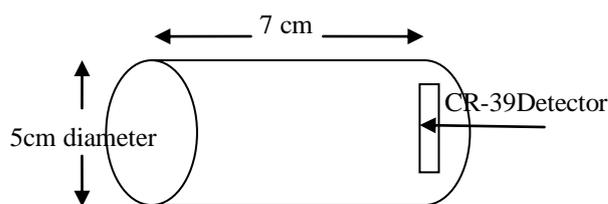
**Fig.(1) Represent the Cup technique used in study subject with CR-39 SSNTD.**
