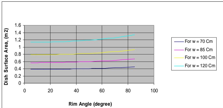
**Figure (4) Solar dish's surface areas versus rim angles for different aperture diameters.**
