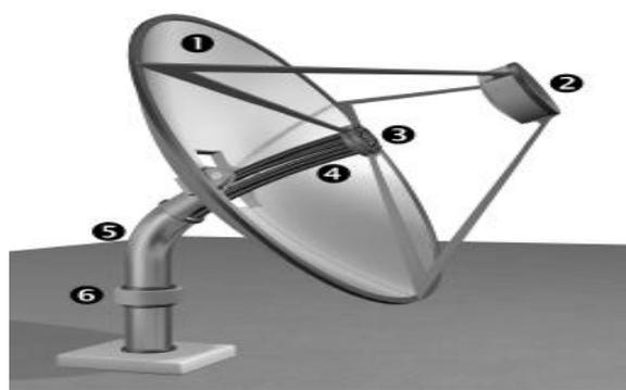
Figure (1) shows solar lighting system, where 1 is primary reflector, 2 is secondary reflector, 3 is fiber mount, 4 is large core optical fiber, 5 is angled stand with altitude tracking mechanism, and 6 is azimuth tracking mechanism [11].
