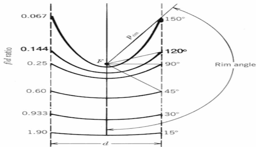
Figure (2) Shows primary reflector (dish) geometrical dimensions [14].
