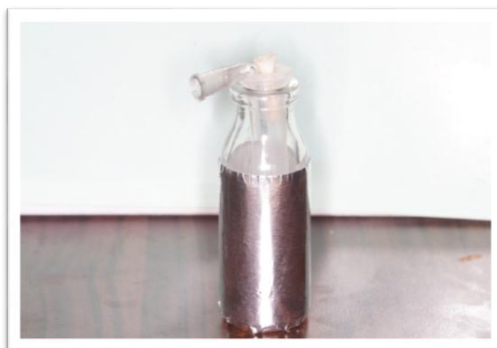
Fig.(1):- Modal system used for evaluation of apical extruded debris.
