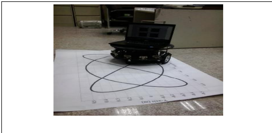
Figure(12). Real set-up experiment of Eddie mobile robot for continuous trajectory tracking.
