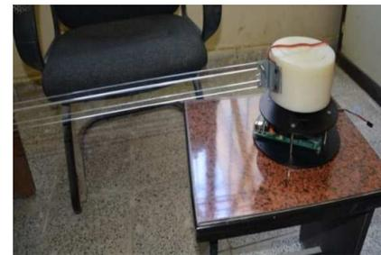
Fig. 4. Flexible link manipulator.
