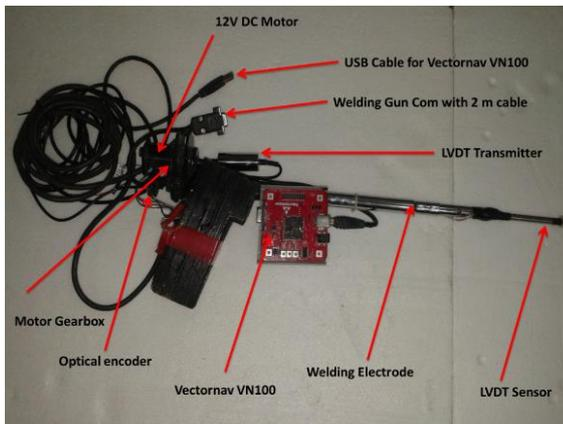
Fig. 3 welding electrode simulator
