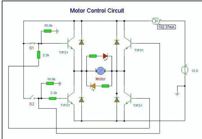
Fig. 5 motor control circuit
