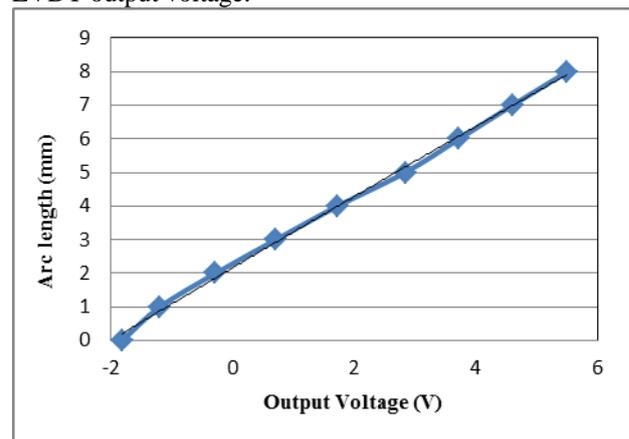
Fig. 7 Relation between welding arc length and output voltage of LVDT sensor.
