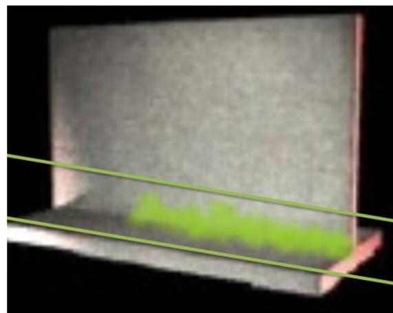
Fig. 4 Two colored parallel lines indicate the recommended arc length
