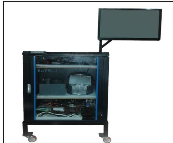
Fig.1 Virtual Welding Training Machine (BasVW 1.1)
