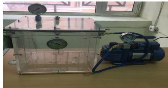
Figure 2: Curing device
