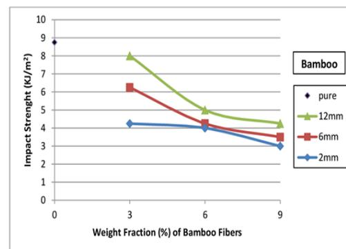
Figure 5: Impact strength of specimens reinforced with bamboo fibers
