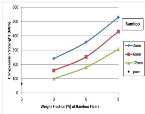
Figure 3: Compression strength of composite specimens reinforced with bamboo fibers.
