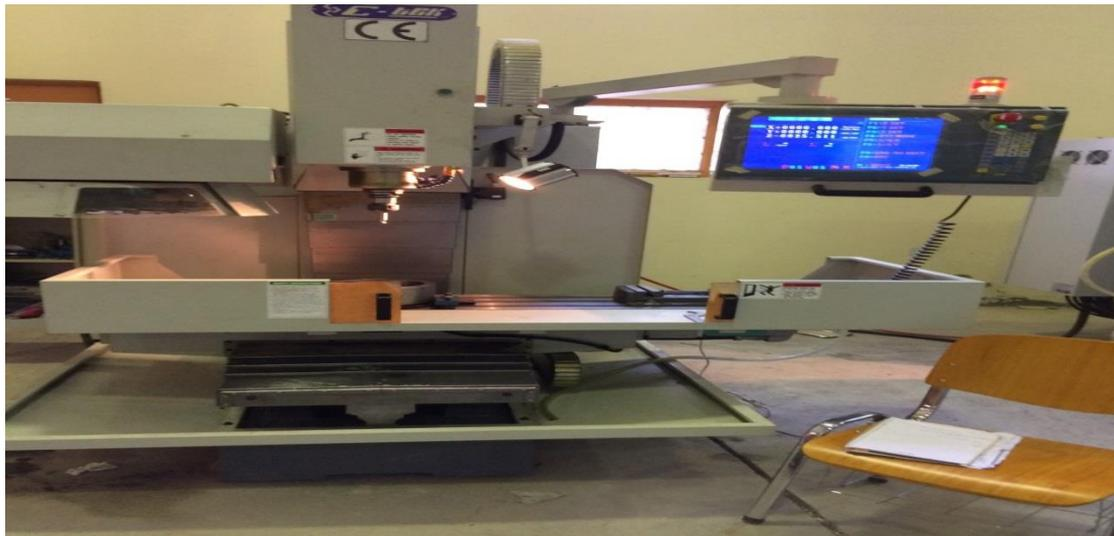
Figure (1) : CNC milling machine used in the experimental work
