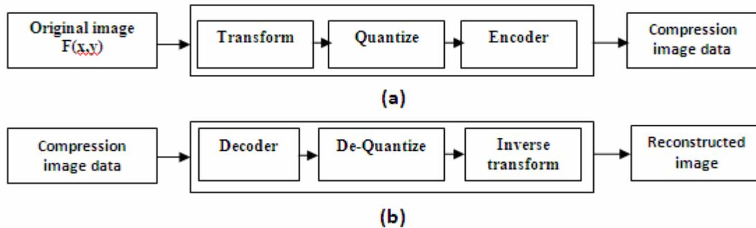
**Fig. 1; Image compression system (a) encoder, (b) decoder.**
