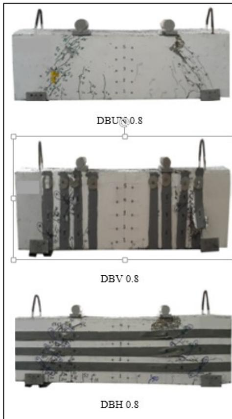
**Figure 11: Failure mode of beam specimens with  $a/d = 0.8$**
