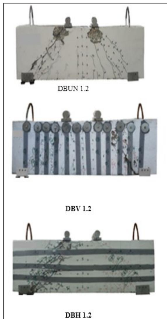
Figure 13: Failure mode of beam specimens with  $a/d = 1.2$
