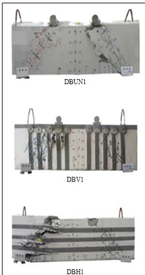
**Figure 12: Failure mode of beam specimens with  $a/d = 1.0$**
