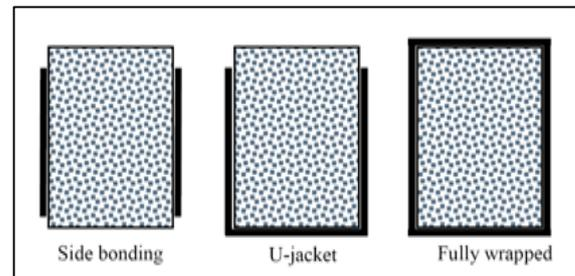
Figure 1: Shear strengthening schemes with FRP composites [8]
