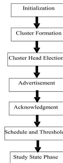
Figure (5): Proposed Static WSN Protocol Structure.
