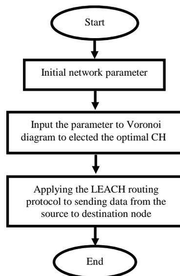
**Figure (2):** Protocol structure representation
