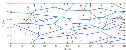
**Figure (11):** Voronoi classification of node sensor.
