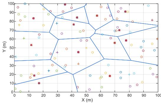
Figure (3): Clustering head selection with Voronoi cells
