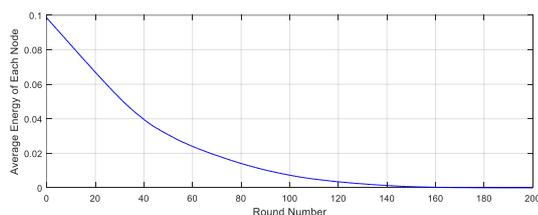
**Figure (13):** Corresponding of average energy of each node.
