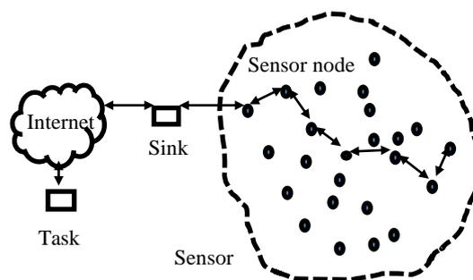
**Figure (1):** A WSN connected to the internet via sink node [1]
