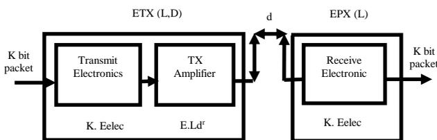
Figure (4): Radio energy dissipation model
