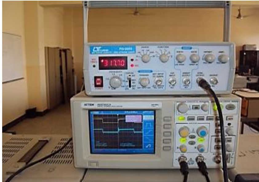
Figure (17): Input and output signal from an oscilloscope with 8QAM.
