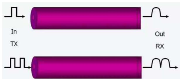
**Figure 5.** Effect of dispersion in optical fiber communication system.
