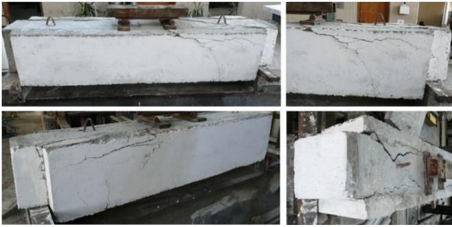
Fig. 12 The (S.-J. + Stirrup) beam after the Testing.
