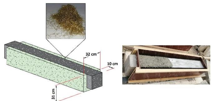
**Fig. 3** Details of the beam (S.-J. + Steel Fiber).
