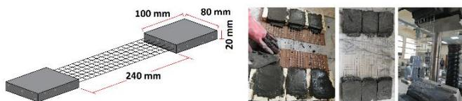
**Fig. 5** Details of wire mesh tensile coupons.
