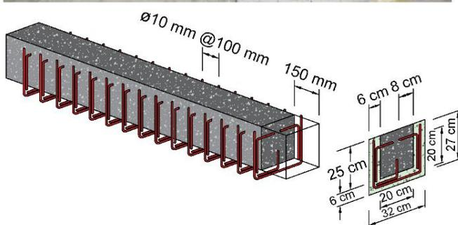
**Fig. 4** Details of the beam (S.-J. + Stirrup).
