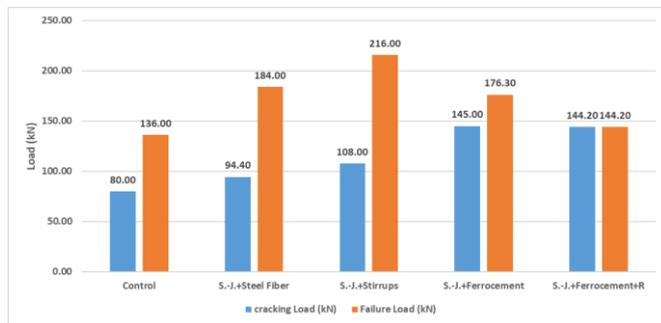
**Fig. 8** The cracking and failure load for all the studied beams.
