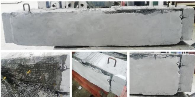
Fig. 13 The (S.-J. + Ferrocement) beam after the failure.
