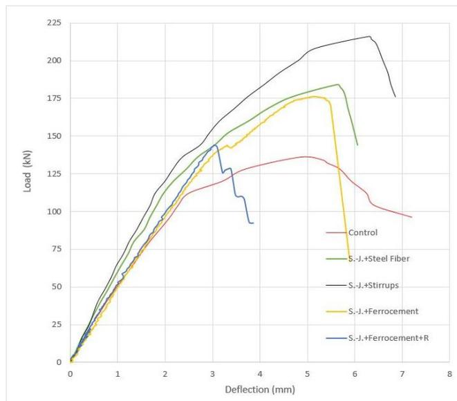
**Fig. 9** The Load-deflection Curves in the Mid-span of Overall Studied beams.
