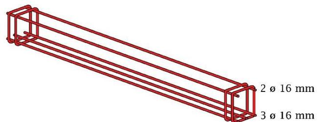
Fig. 2 Reinforcement details.
