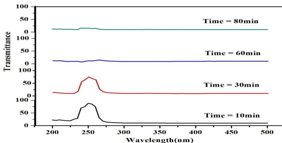
**Fig (3) UV-Visible spectrum for PMMA membranes treated by (42W), SF<sub>6</sub>-plasma.**
