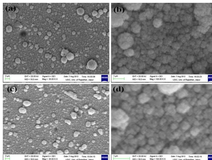
**Fig (2) SEM micrographs of PMMA film treated by (42W), SF<sub>6</sub>–Plasma (a) 20kX- mag. for (30 min) treatment, (b) 100kX- mag. for (30 min) treatment, (c) 20kX-mag. for (80 min) treatment and (d) 150kX-mag. for (80 min) treatment.**
