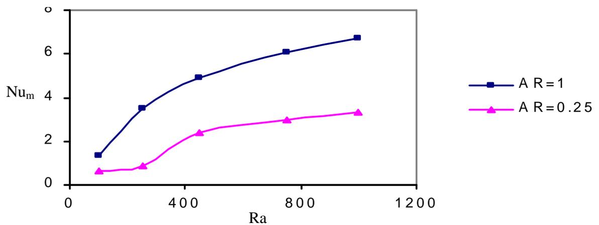
**Fig.10** Variation of the mean Nusselt number with Rayleigh number for the square enclosure AR=1 and the trapezoidal enclosure AR=0.25 .
