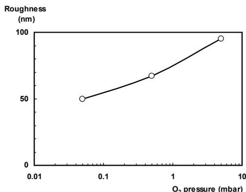
**Fig. (2) Dependency of surface roughness of ZnO thin films prepared by PLD on the O<sub>2</sub> pressure inside the deposition chamber**
