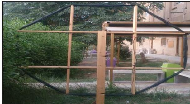
Figure 2. Octagonal antenna of wood at the monitoring station of the Faculty of Science, Thi-Qar University.
