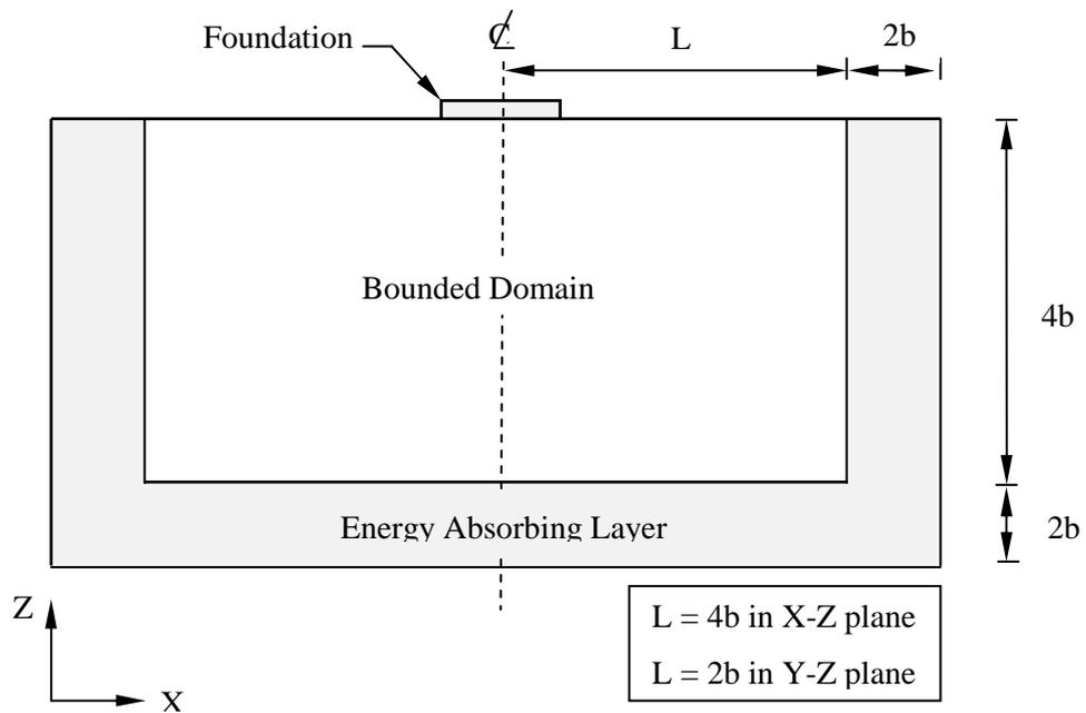
Figure (2): Basic features of the numerical model using energy absorbing layer.
