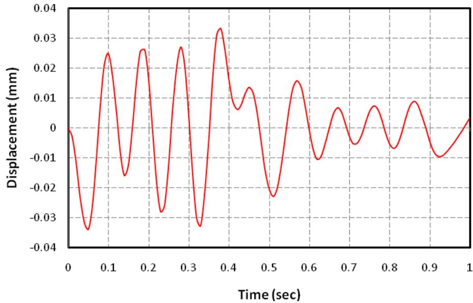
Figure (6): Displacement of the foundation at point A using elementary boundaries.
