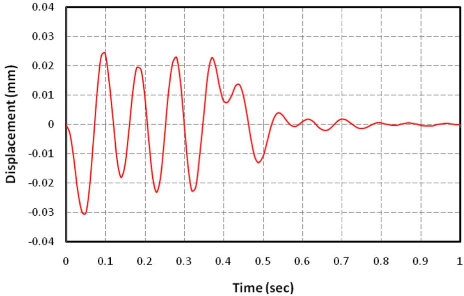
Figure (8): Displacement of the foundation at point A using energy absorbing layer.
