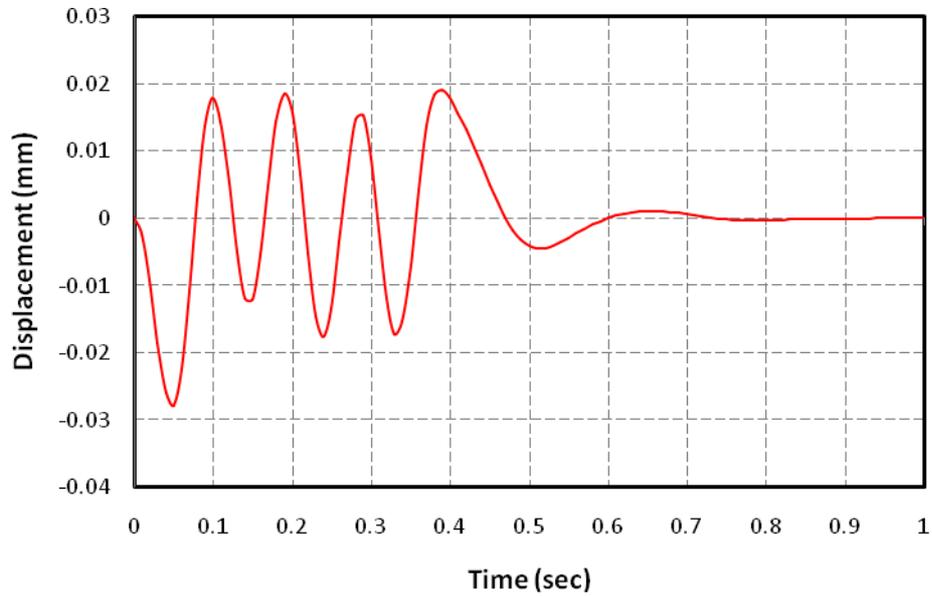
Figure (10): Displacement of the foundation at point A using energy absorbing layer with material damping.
