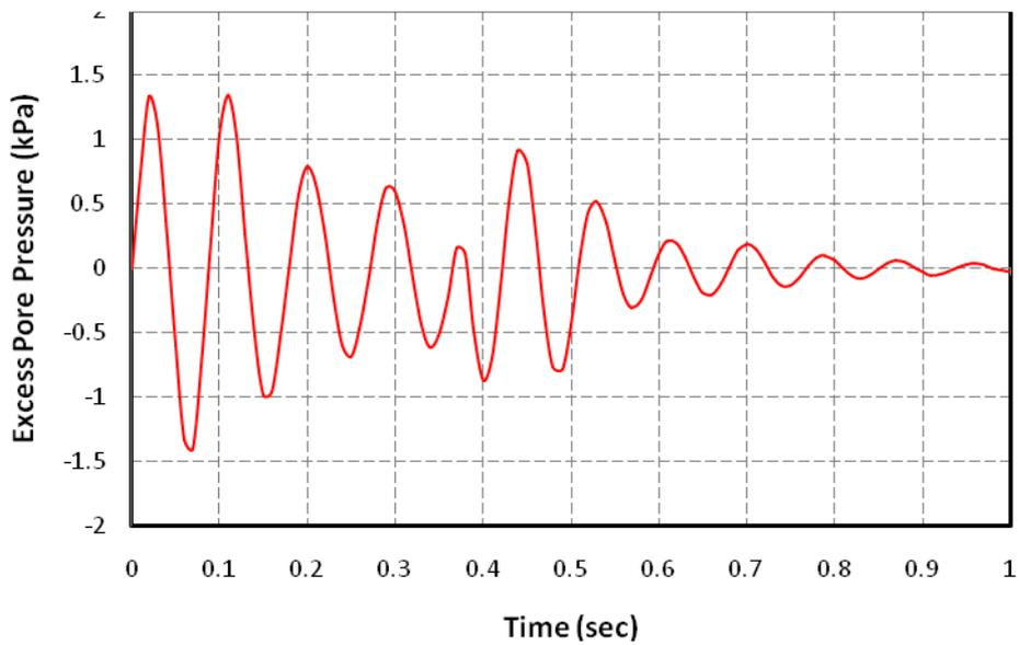
Figure (9): Excess pore water pressure at point A using energy absorbing layer.
