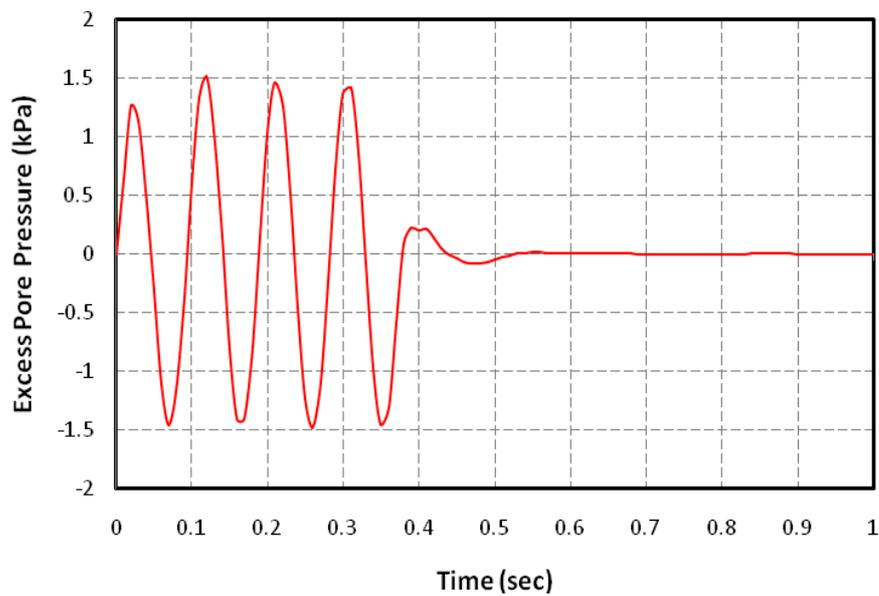
Figure (11): Excess pore water pressure at point A using energy absorbing layer with material damping.
