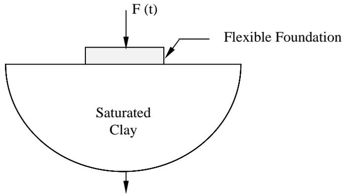
Figure (3): Elastic foundation on a semi-infinite saturated clay.
