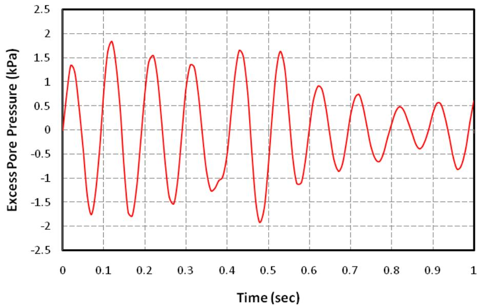
Figure (7): Excess pore water pressure at point A using elementary boundaries.
