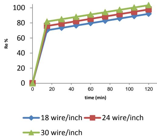
Fig. 7. Effect of mesh number on Mn Re % at initial Mn conc. = 100 ppm and C.D. = 40 mA/cm<sup>2</sup>
