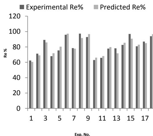
Fig. 2. Comparison between Experimental and predicted Re% values of Mn removal
