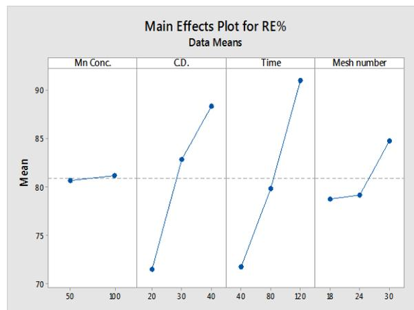
Fig. 3. Main effect plot for means values of Re% for Mn removal
