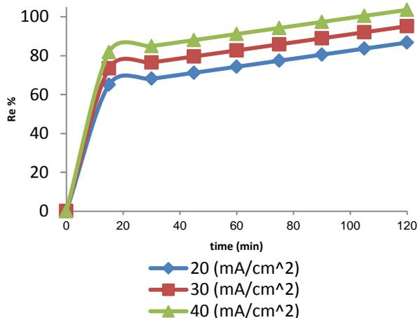
Fig. 6. Effect of C.D. on Mn Re % at initial Mn conc. = 100 ppm and mesh number = 30 wire/inch
