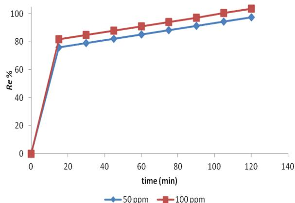
Fig. 5. Effect of initial Mn Concentration on Mn Re% at C.D. = 40 mA/cm<sup>2</sup> and mesh number = 30 mm
