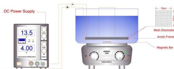
Fig. 1. A schematic photo of ECF cell
