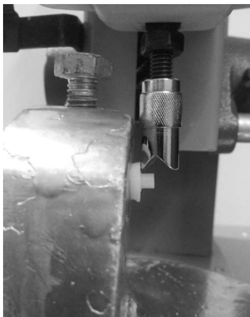
Figure (2): sample was fixed on universal testing machine for shear test.
