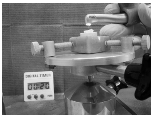
Figure (1): Laser irradiation of dentin surface by Waterlase iplus, laser handpiece and sample were fixed on survivor for parallism.
