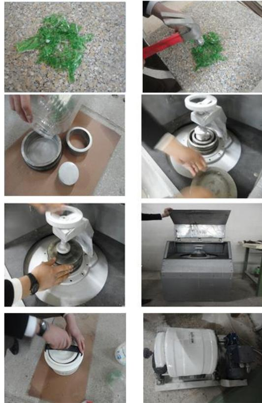
Figure (3): Stages of glass grind
