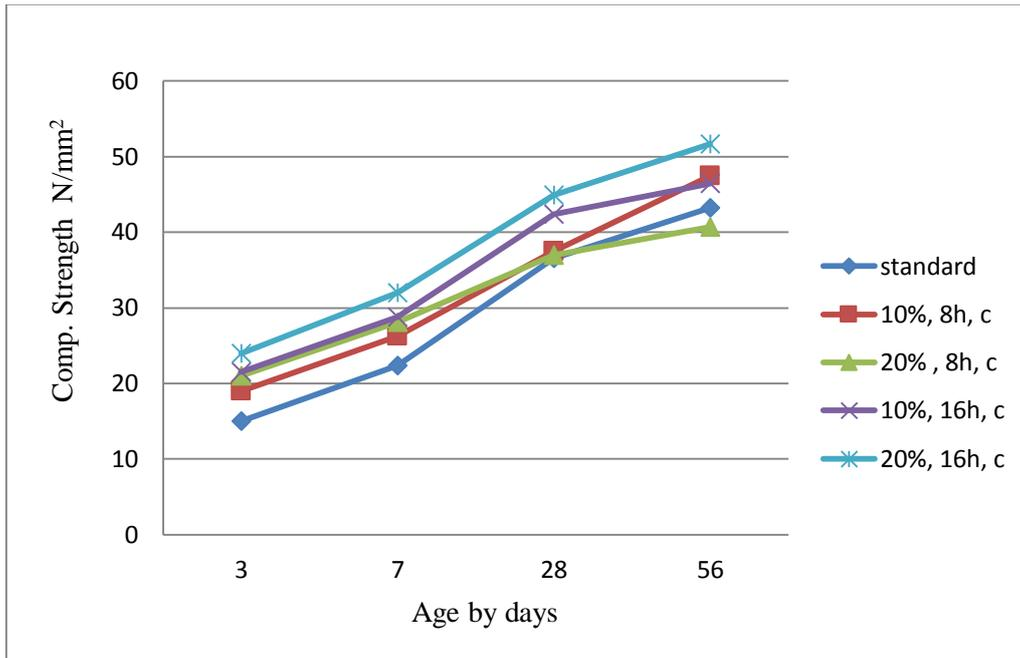
Figure (5): Compressive strength for standard samples and the samples which contain the ratios of glass powder instead of cement.
