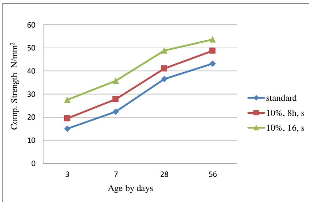
Figure (6): Compressive strength for standard samples and the samples which contain the ratios of glass powder instead of sand.
