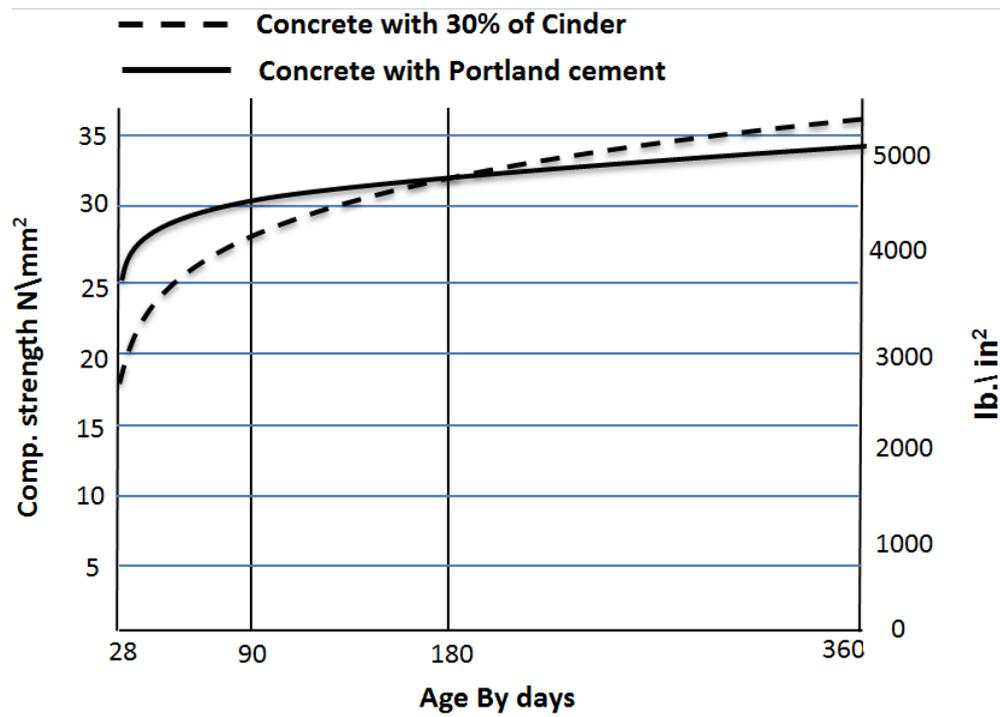
Figure (7): Effects of compensation pazzolanic materials as a part of the cement on the compression strength of concrete.
