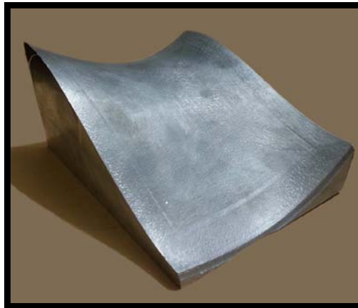
Fig.(6): The specimen implemented in the Workshops and Training Center in the University of Technology /Iraq- Baghdad using C-TEK CNC milling machine.
