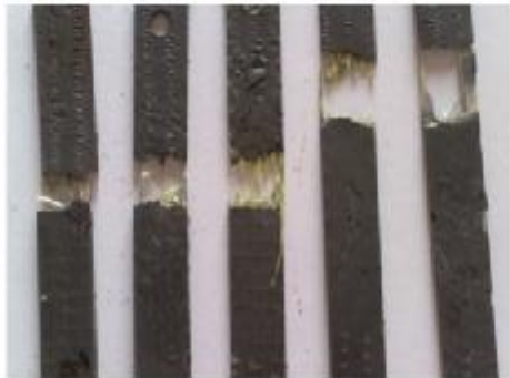
Figure (10) Shows the fracture regions for (EAKG, EAKPVC and EAGPVC) samples
