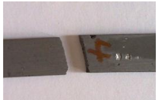
Figure (3) Shows the fracture region for (EA) sample.
