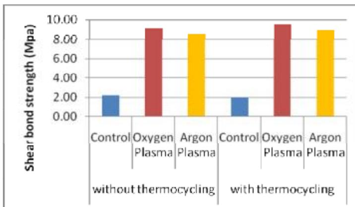
**Figure 1: SBS in (Mpa) of all experimental groups with and without thermocycling.**
