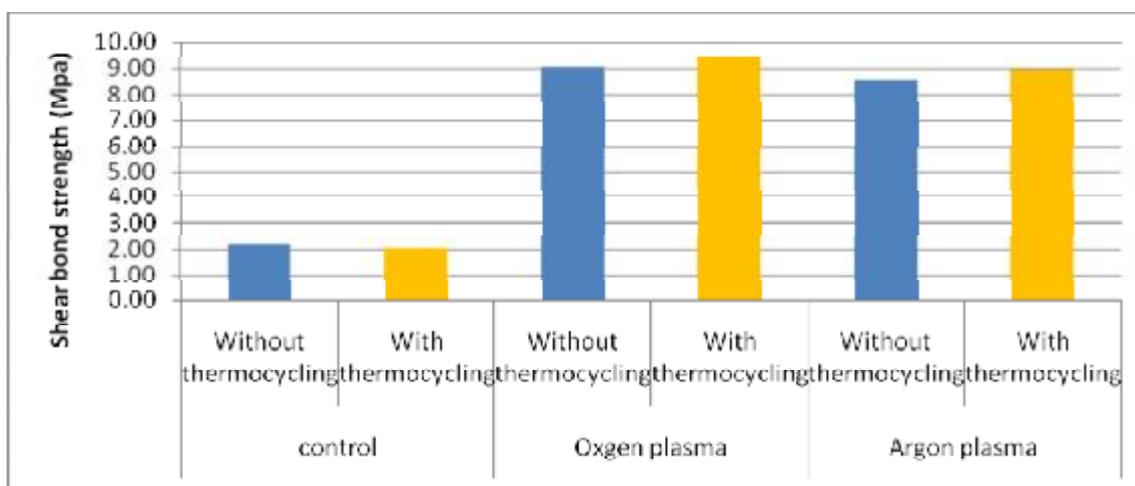
**Figure 2: Comparison of the effect of thermocycling on SBS in (Mpa) in each experimental group.**
