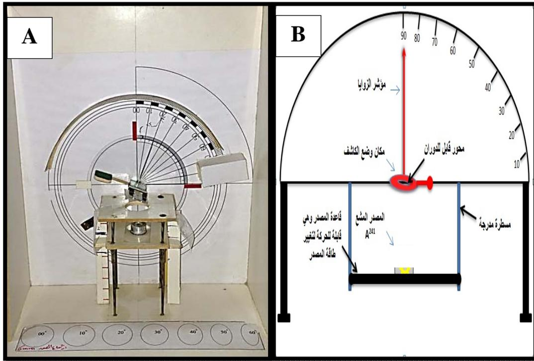
**Fig. 1: (A) System of irradiation at different angles, (B) Scheme of irradiation system at different angles**
