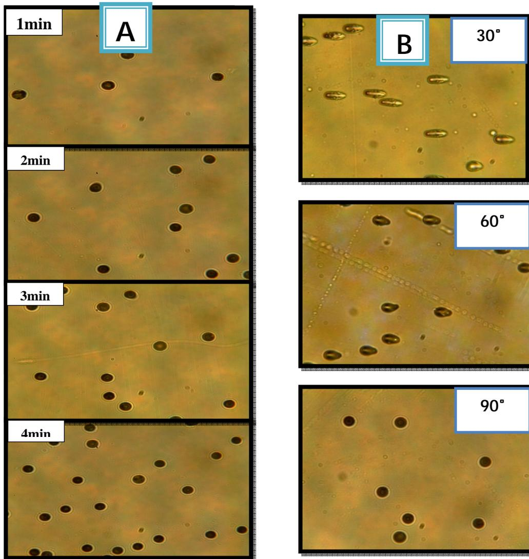
**Fig. 2: Samples of images of tracks taken by the digital camera (A): for different irradiation times, (B): for different incidence angles**
