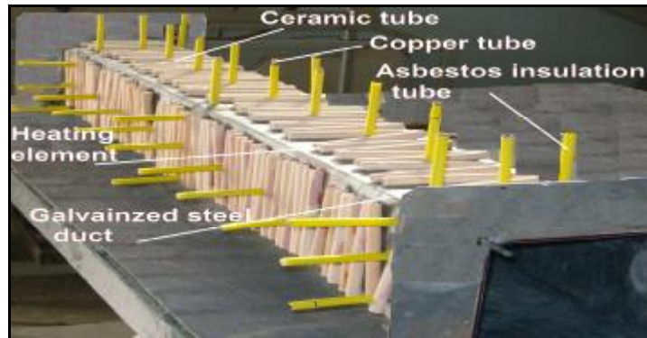
Figure (4) Heating arrangement on test duct
